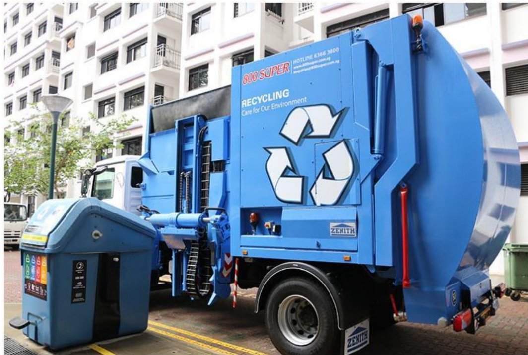
Figure 2: Side loader with a robotic lifting arm attached to the side of the truck
